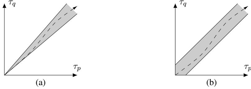
Figure 13. Bounding the clock drifts by ratio and difference
