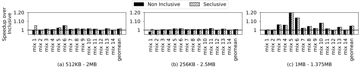
Fig. 3. Performance improvement in SPEC 2017 mixes in an 8-core system with different L2-LLC cache sizes.(higher the better).
