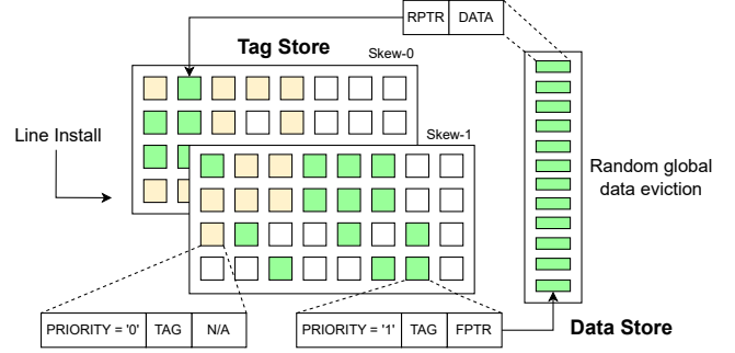
Fig. 3: Overview of the Maya cache design. White blocks represent invalid tag entries, yellow represents priority-0 tag entries, and green represents priority-1 tag entries.
