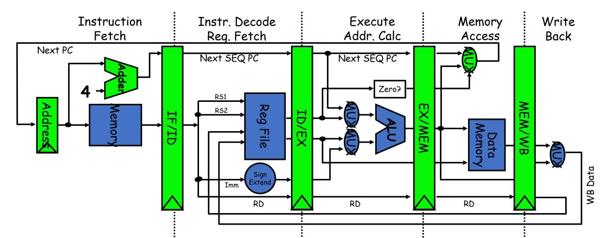
The right place to put the MUX that selects PC+4 and the target is the fetch stage. The slide shows a vanilla 5-stage pipeline if we just take a single cycle datapath and divide it into five stages. Computer Architecture
