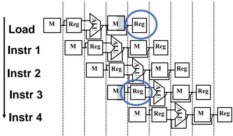
Can read/write the register file (same register) in same clock cycle ⓒ but.. Real picture is different
