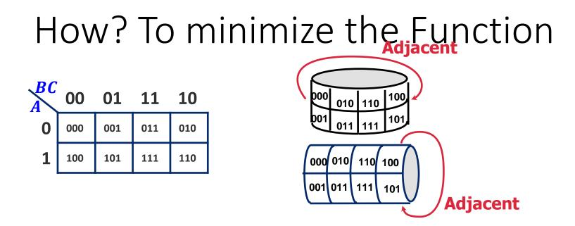
K-map adjacencies go "around the edges" Wrap around from first to last column Wrap around from top row to bottom row
