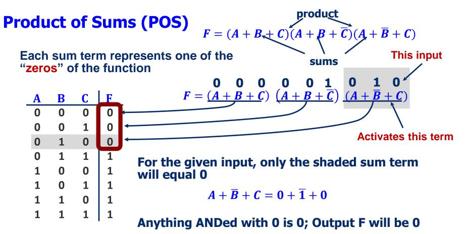
The function evaluates to FALSE (i.e., output is 0) if **any** of the Sums (maxterms) causes the output to be 0 Computer Architecture
