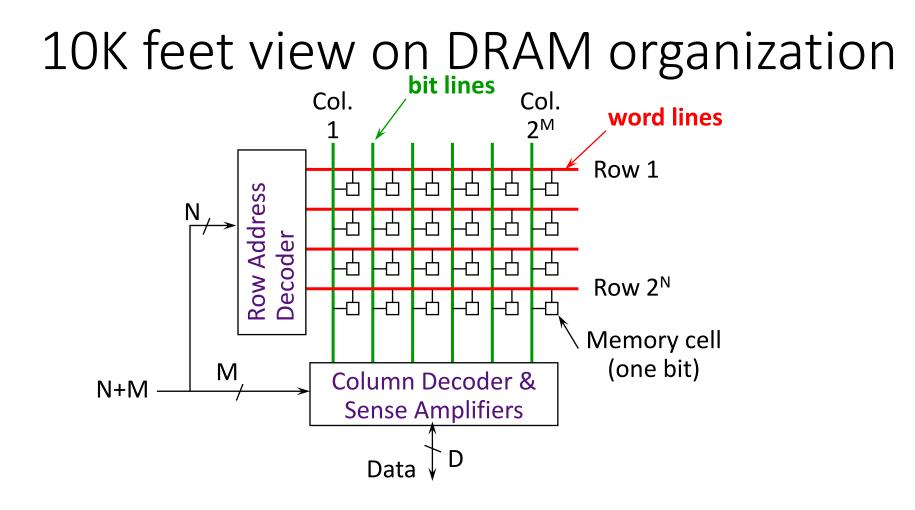
Bits stored in 2-dimensional arrays on chip
