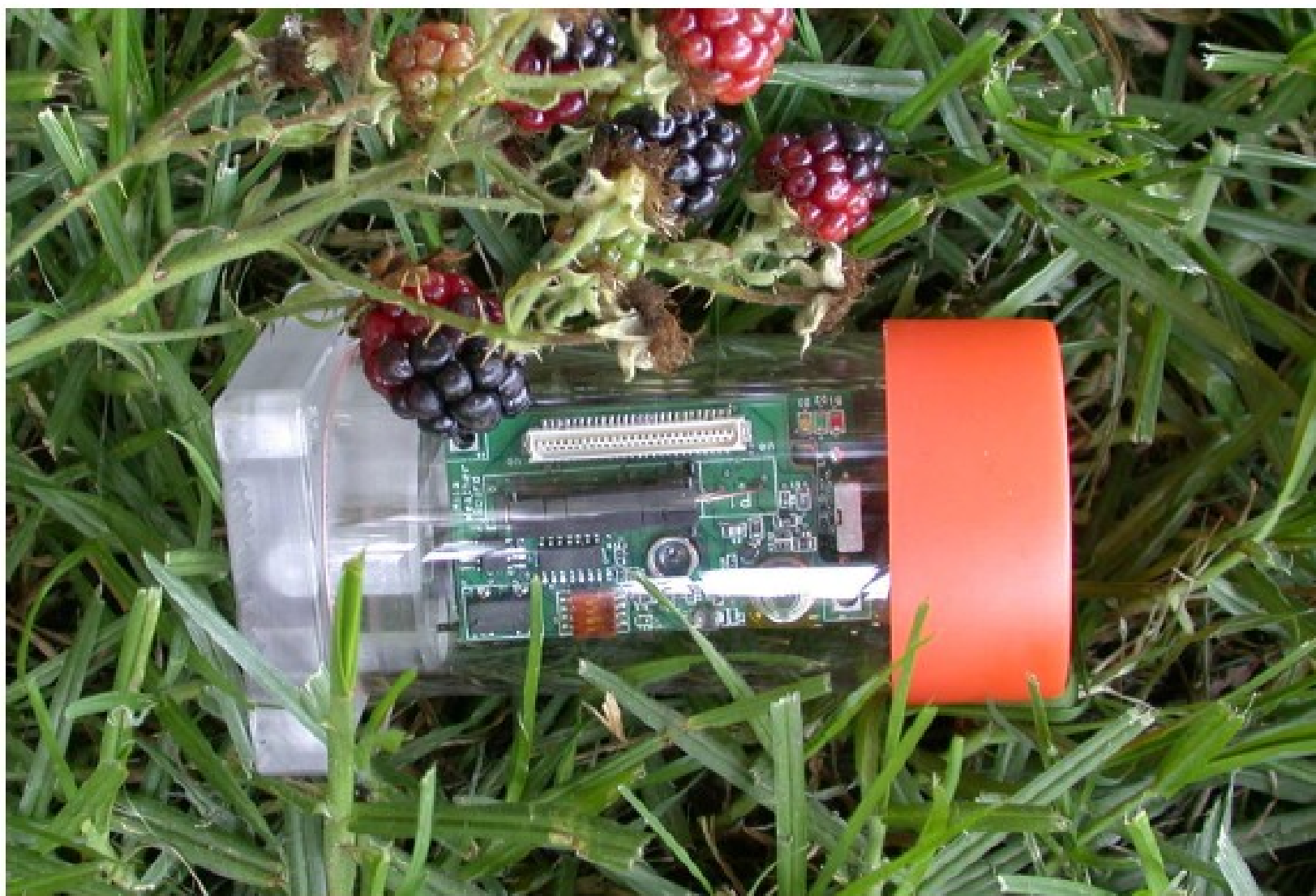
Figure 3: Acrylic enclosure used for deploying the Mica mote.
