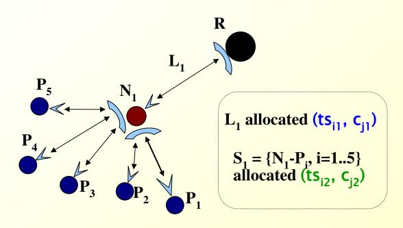
At most <u>two channels</u> for long-distance links at <u>hop-1</u> nodes Only <u>one channel</u> for long-distance link at <u>hop-2</u> nodes
