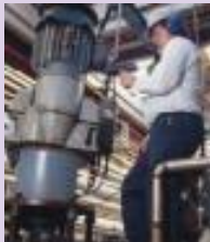
Monitoring bearings with the Ultraspote.
