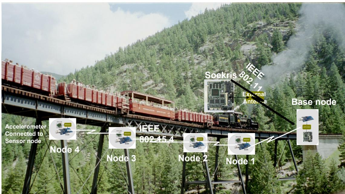
Figure 1.1: Schematic description of our solution at work along with the problem setting
