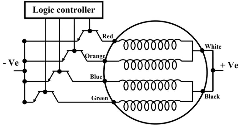
Figure 3.8: Stepper Motor circuit
