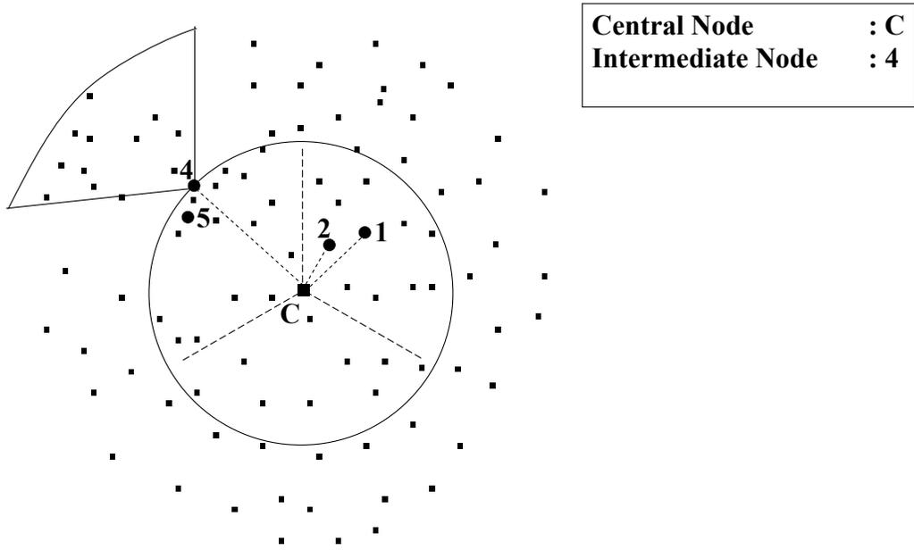
Figure 1.2: Long Distance Network with sector antennae at node C and directional antennae at nodes 1 and 2.
