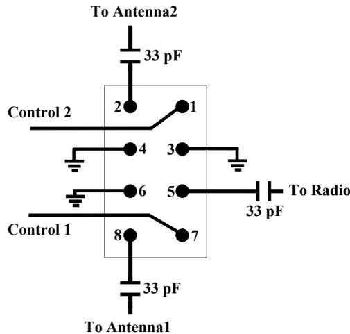
Figure 3.3: RF-Switch with PSW-1211
