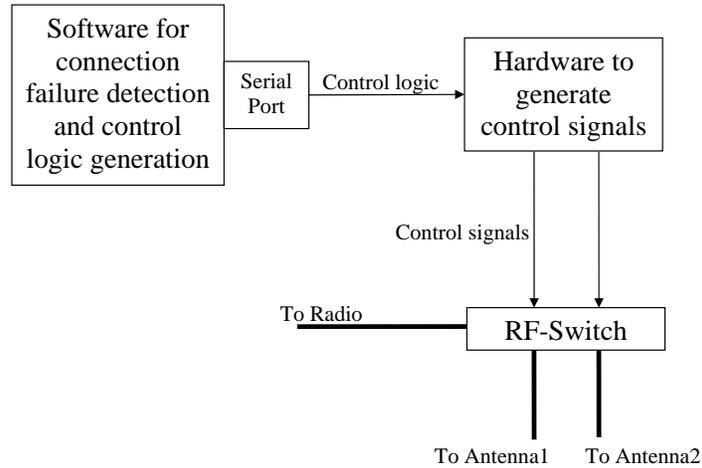
Figure 3.2: Block diagram of Replication solution
