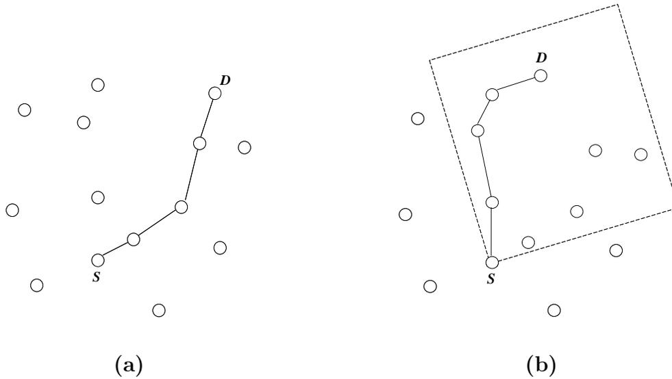
Figure 2.2: Ad-hoc Network with directional antennae
