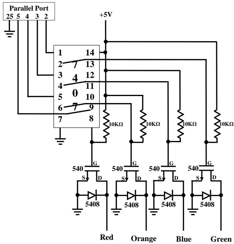
Figure 3.9: Circuit for stepper motor
