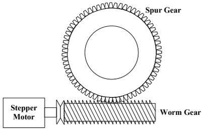
Figure 3.11: Spur Gear and Worm Gear
