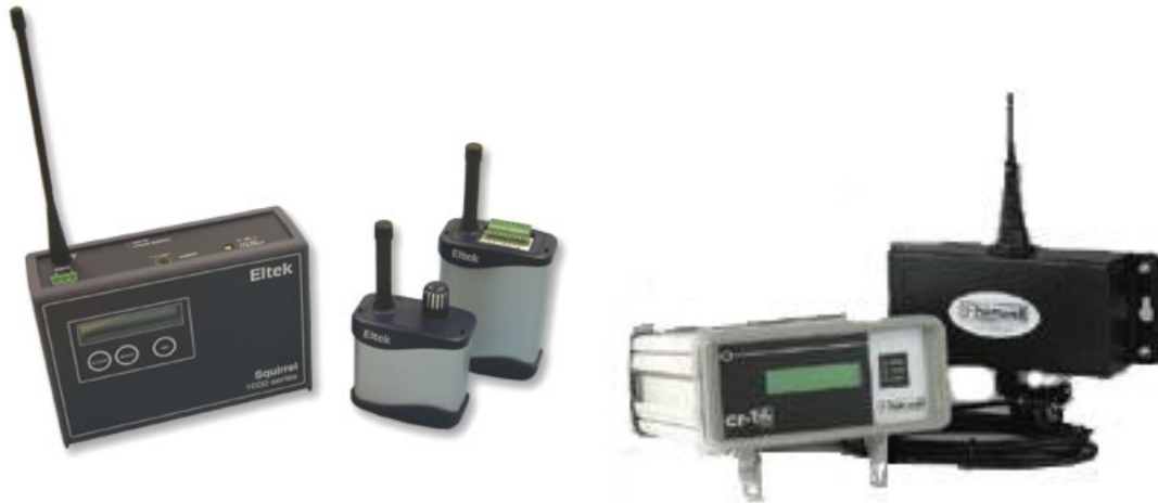
Figure 1.4 Single hop wireless data logging solution (Source: www.eltekdataloggers.co.uk , www.seaworthsys.com/industrial_internet/hanwell )
