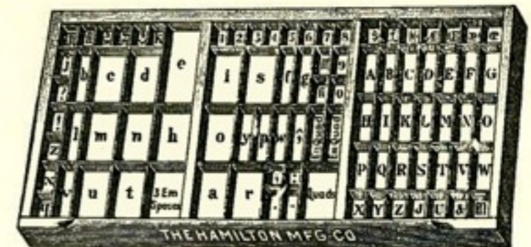
California Job Case. FIG. 2.—Showing Lay of Cases.
