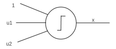
Let the desired output be 1 when elements of class  $A = \{(1,2),(2,4),(3,3),(4,4)\}$  is applied as input and let it be -1 for the class  $B = \{(0,0),(2,3),(3,0),(4,2)\}$ . Let the initial connection weights  $w_0(0) = +1, w_1(0) = -2, w_2(0) = +1$  and learning rate be h = 0.5.
