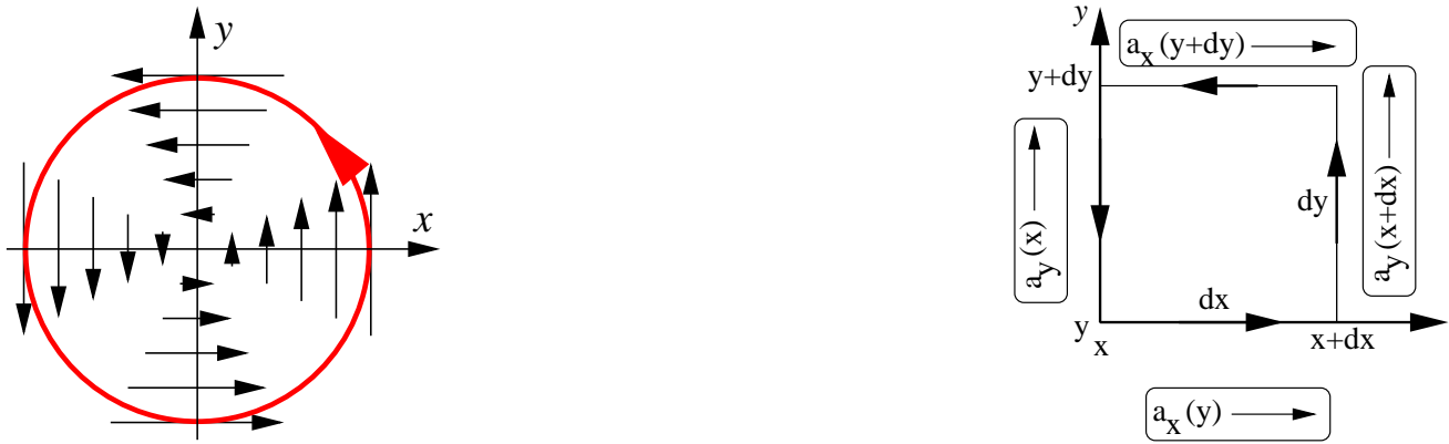
Figure 5.5: (a) A rough sketch of the vector field -y\hat{i} + x\hat{j} . (b) An element in which to calculate curl.
