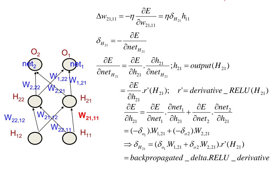
$\Delta W_{21,11} = \eta[(t_2 - o_2)W_{2,21} + (t_1 - o_1)W_{1,21}] \cdot r'(H_{21}) \cdot h_{11}$
