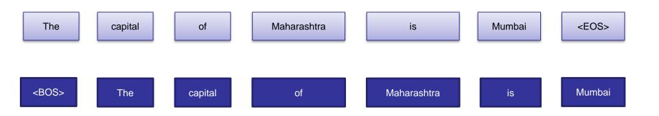
The output sequence is one-time step ahead of the input sequence
