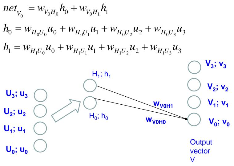
Developing "net<sub>vi</sub>" (2/2) • For "heavy", only  $u_0$  is 1,  $u_1 = u_2 = u_3 = 0$ • So,  $h_0 = w_{H_0 U_0}$  $h_1 = W_{H_1U_0}$  $net_{v_0} = w_{V_0H_0}w_{H_0U_0} + w_{V_0H_1}w_{H_1U_0}$  $= \begin{bmatrix} w_{H_0U_0} & w_{H_1U_0} \end{bmatrix} \begin{vmatrix} w_{V_0H_0} \\ w_{V_0H_1} \end{vmatrix}$
