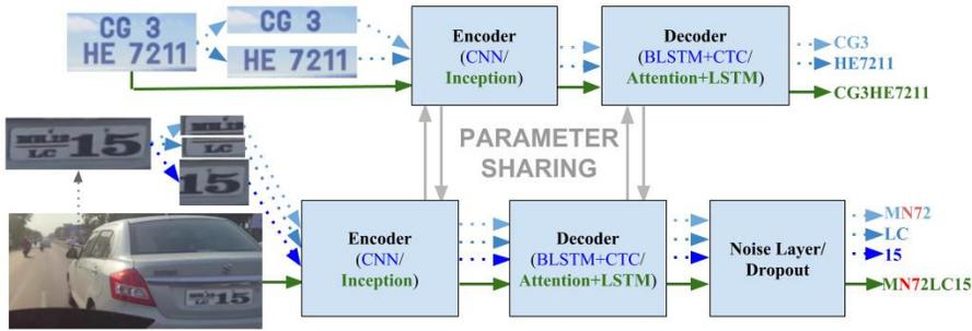
Fig. 3. We train our models on synthetic clean data (top) & real noisy labeled data (bottom). The license plate image flows in multiple splits through the *baseline model*, shown by dotted blue arrows. For the *end-to-end model*, the entire image flows through the model together, shown by green arrows.
