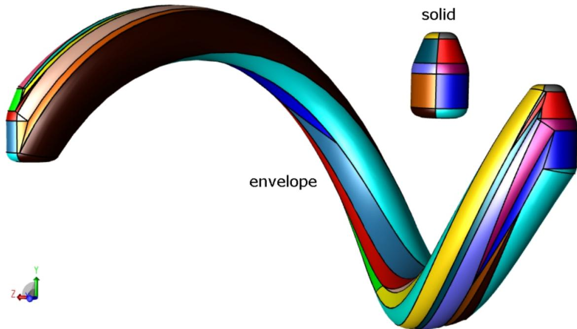
Figure: A simple bottle being swept along a screw motion with compounded rotation. Correspondence between faces of  $\partial M$  and those of the envelope is shown by color coding.
