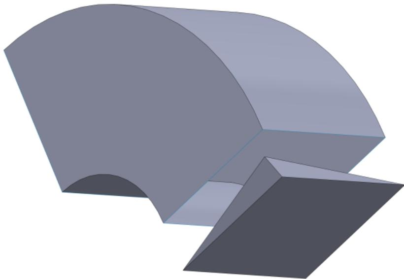
Figure: A pyramid swept along a curvilinear trajectory
