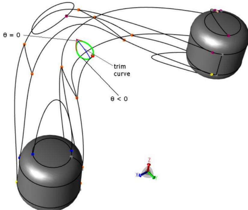
Figure: Example of a non-decomposable sweep: a cylinder being swept along a cosine curve in  $xy$ -plane while undergoing rotation about  $x$ -axis. The curve  $\theta = 0$  is shown in red and trim curve is shown in blue. The portion of the swept edges where  $\theta$  is negative is shown in green.
