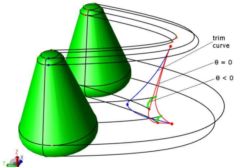
Figure: Example of a non-decomposable sweep: a cone being swept along a parabola. The curve  $\theta = 0$  is shown in red and trim curve is shown in blue. The portion of the swept edges where  $\theta$  is negative is shown in green.
