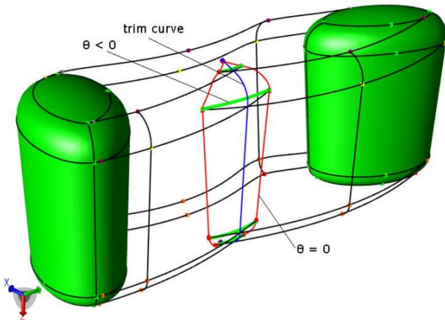
Figure: Example of a non-decomposable sweep: an elliptical cylinder being swept along  $y$ -axis while undergoing rotation about  $z$ -axis. The curve  $\theta = 0$  is shown in red and trim curve is shown in blue. The portion of the swept edges where  $\theta$  is negative is shown in green.
