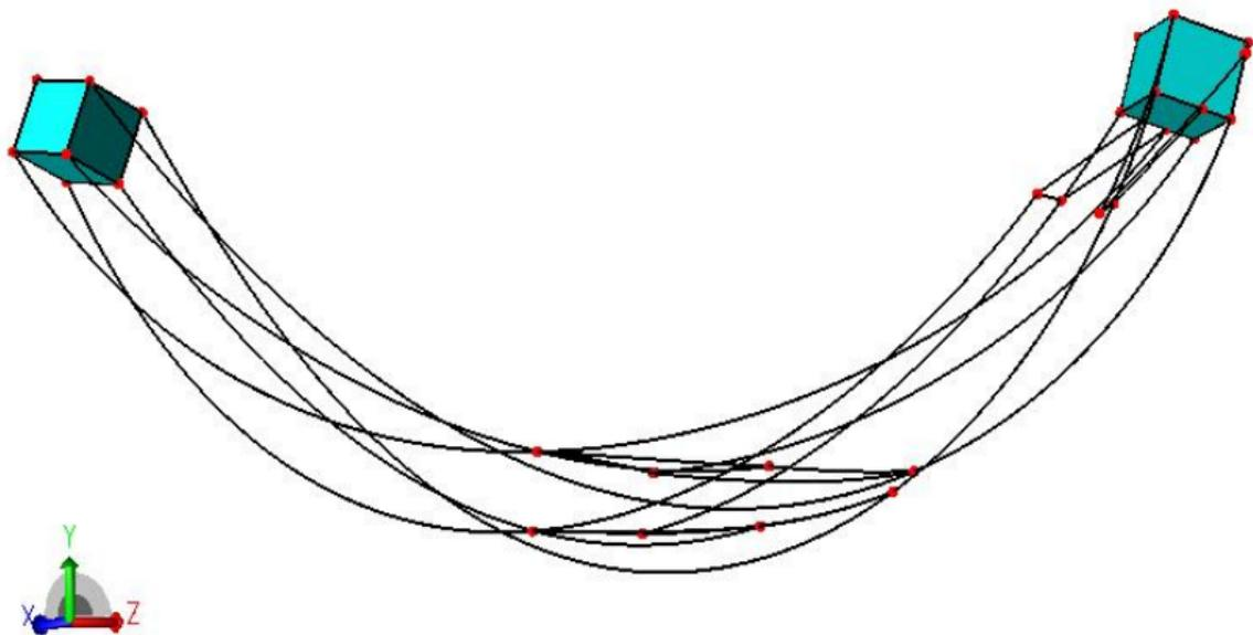
Figure: The 1-cage of the envelope obtained by sweeping a cube.
