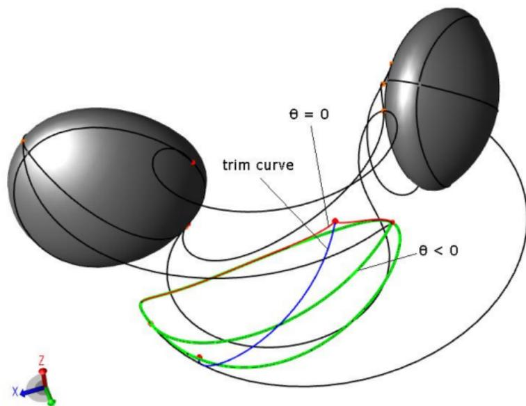
Figure: Example of a non-decomposable sweep: a blended intersection of a sphere and an ellipsoid being swept along a circular arc in  $xy$ -plane while undergoing rotation about  $z$ -axis. The curve  $\theta = 0$  is shown in red and trim curve is shown in blue. The portion of the swept edges where  $\theta$  is negative is shown in green.
