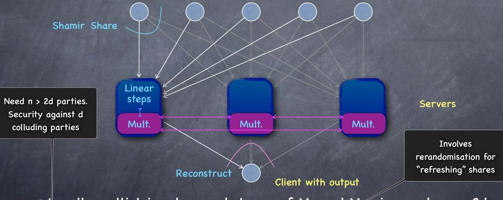
Locally multiplying degree d shares of M<sub>1</sub> and M<sub>2</sub> gives a degree 2d share of M<sub>1</sub>·M<sub>2</sub>. Then securely switch back to a degree d share (involves communicating degree d shares of degree 2d shares)
