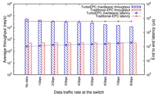
Figure 15: TurboEPC throughput with data traffic interference.
