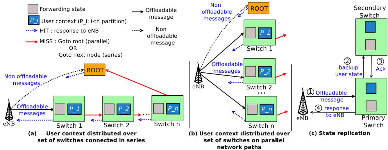
Figure 4: Scalability and fault tolerance in TurboEPC.
