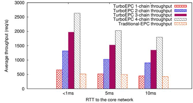
Figure 9: Throughput with varying distance to core, and varying number of dataplane switches.
