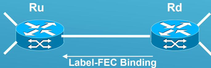
Unsolicited Downstream Label Distribution
