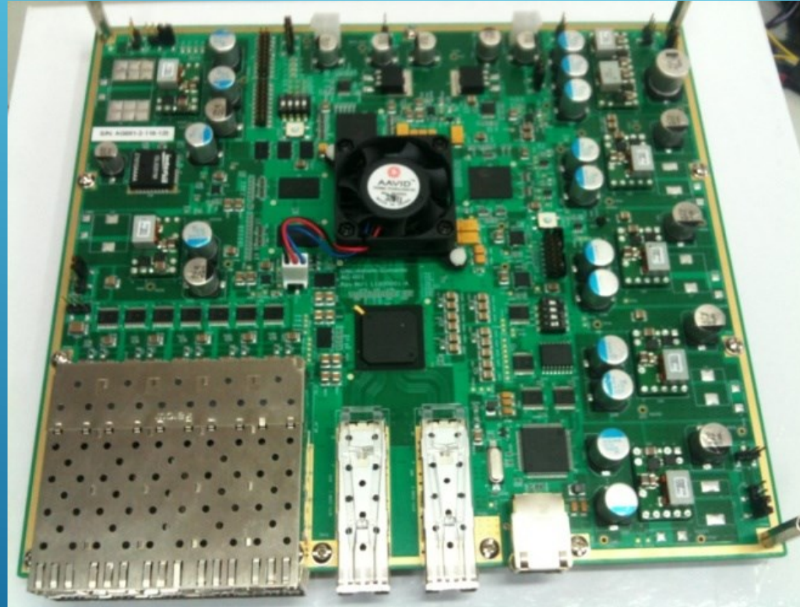
Fig 1. The Carrier Ethernet Switch Router(CESR) hardware
