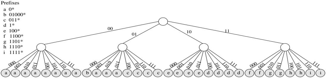
Figure 16: A two level full expanded multibit trie
