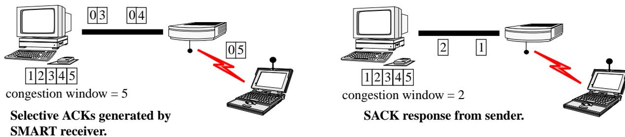
**Figure 3. TCP with SMART-based selective acknowledgements**
