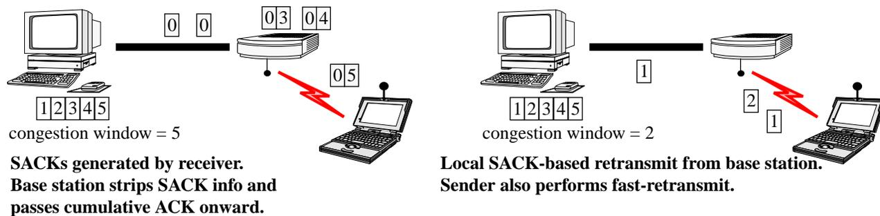
Figure 6. Link-Layer with SMART-based selective acknowledgments
