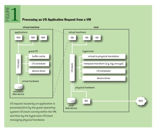
presented with the illusion of having its own dedicated virtual hardware, in reality the hypervisor must multiplex limited physical hardware across multiple VMs of varying importance, mapping their virtual resources onto available physical resources. At the most basic level, contention for a physical device will result in scheduling delays for some VMs. At a minimum, the hypervisor must prevent VMs from monopolizing resources and denying service to others.
