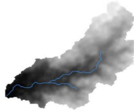
c) Stream network is generated from clipped Raster layer
