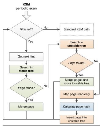
**Figure 4.** The high-level workflow of our hinting mechanism. For every hint we process, we first check if a merge partner can be found in either the stable or in the unstable tree. If we find a match, we merge the pages in the same way KSM does. Otherwise, we remap the page read-only (if it is not already), calculate its hash-value and insert it into the unstable tree. When all hints have been processed before the scan rate is exceeded, we continue with the regular KSM scan path.
