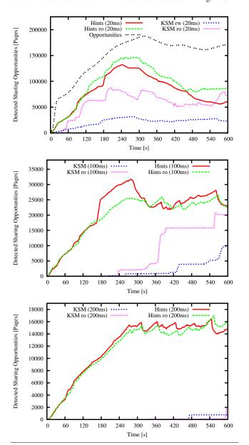
**Figure 8.** Kernel build merge performance at 100 pages per wake-up with varying wake-up times. Top to bottom: 20 ms, 100 ms, 200 ms. The first graph also shows the theoretical maximum of sharing opportunities that could be exploited.
