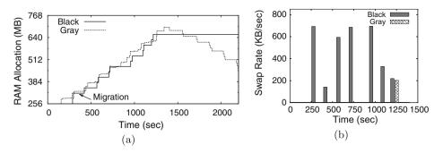
Fig. 6. The black-box system lags behind the gray-box system in allocating memory. The gray-box approach proactively increases memory and safely reduces the VM's memory allocation when demand falls.
