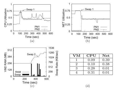
Fig. 5. Swaps and migrations to handle network- and memory-intensive loads. Initially, VM<sub>1</sub> and VM<sub>2</sub> are on PM<sub>1</sub>, the rest on PM<sub>2</sub>. After two swaps, PM<sub>1</sub> hosts VM<sub>1</sub> and VM<sub>4</sub>.
