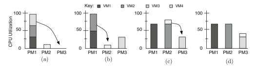
Fig. 7. The black-box system incorrectly guesses resource requirements since CPU usage is saturated, resulting in an increased resolution time. The graybox system infers usage requirements and transitions directly from (a) to (d).
