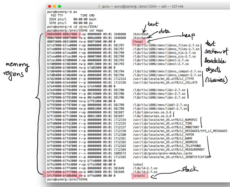
Figure 2.1: Memory regions and components of a process as shown on a Linux system.
