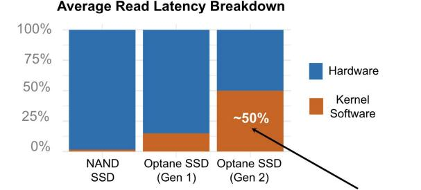
Kernel software overhead accounts for ~50% of read latency on Optane SSD Gen 2
