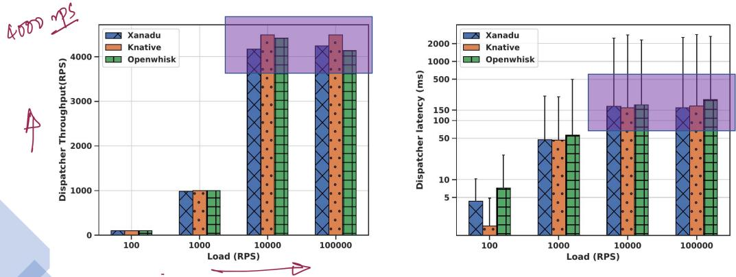
Userspace dispatchers saturate at moderate loads (with high dispatch latency)
