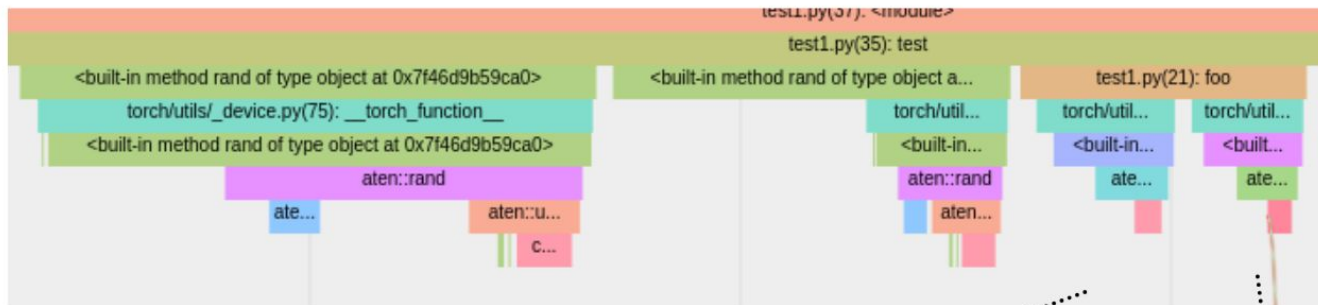
Figure 1: High level Profile Capture. The 2 aten::rand calls are the data preparation done before the function foo is called.
