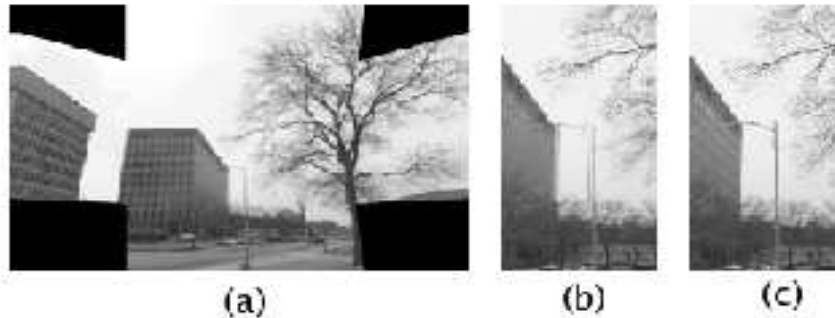
Figure 2.1: Part(a) shows one image of a hemispherical tiling blended with its adjacent images. Part(b) illustrates blurring due to incorrect pose estimates. Part(c) shows the same view after optimization.
