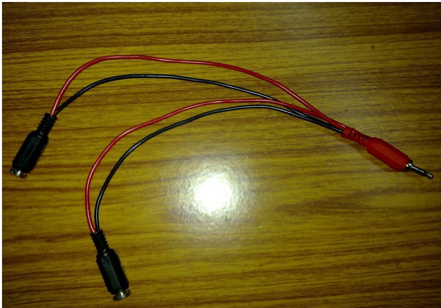
audio connector, two mono inputs, one stereo output (8 solder points)
