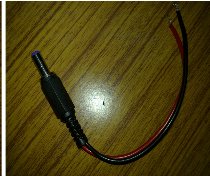
power to GPRS modem from interfacing PCB (2 solder points)
