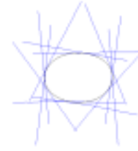
Figure 7: Cross section plane contours and a fitted cross section curve
