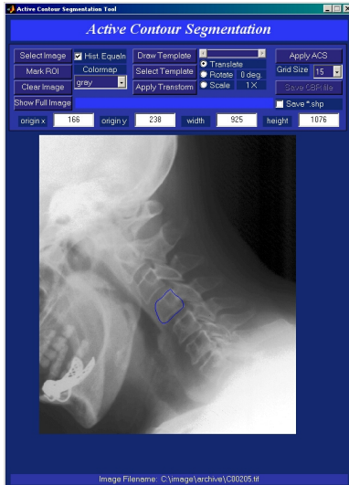
Figure 3: Active Contour Segmentation Tool: Main Window
