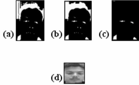
Figure 3: (a) Thresholded image  $B$ . (b) Image after morphological operator applied to  $B$ . (c) Image after region filtering. (d) Detected face resized to 50x50 pixels after template matching.
