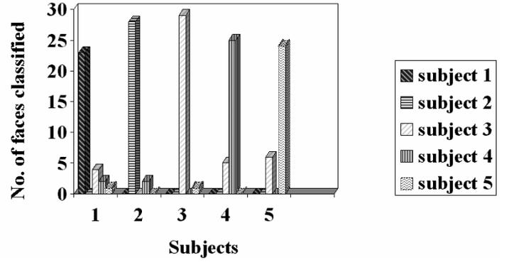
Figure 7: Face recognition performance. The bar graph shows the number of faces classified out of 30 test face patterns for each subject
