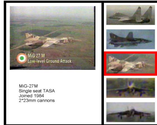
Figure 7: Proposed interface for video-object hyperlinking and virtual annotation. When a video object appears, the corresponding annotation appears below it, and possible hyperlinks are highlighted in the sidebar on the right.
