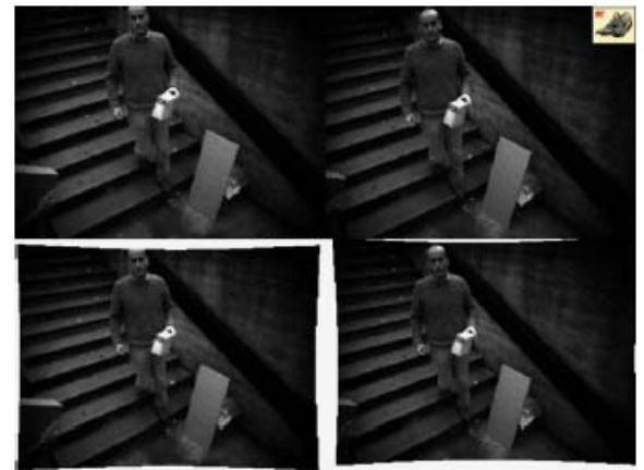
Figure 3. Frame 211 of the "OutdoorZoom" stereo sequence. (Top Left) Original Left Image, (Top Right) Original Right Image, (Bottom Left) Rectified Left Image, (Bottom Right) Rectified Right Image
