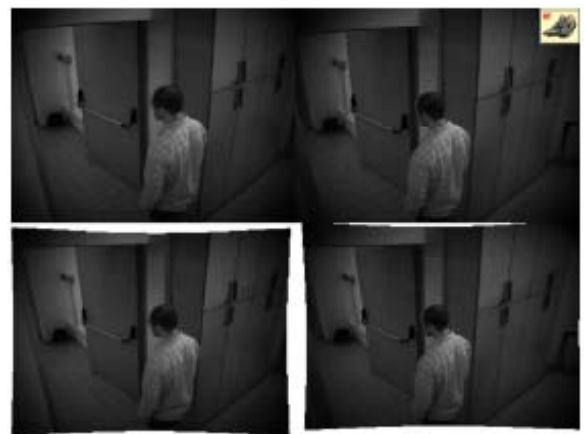
Figure 5. Frame 53 of the "IndoorZoom" stereo sequence. (Top Left) Original Left Image, (Top Right) Original Right Image, (Bottom Left) Rectified Left Image, (Bottom Right) Rectified Right Image
