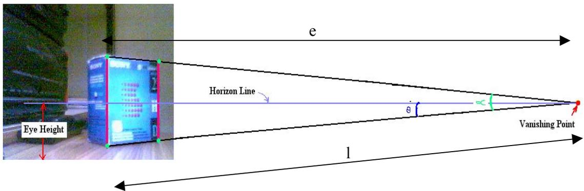
Fig. 2.6: The Image taken and the edges dimensions being calculated using the above method.
