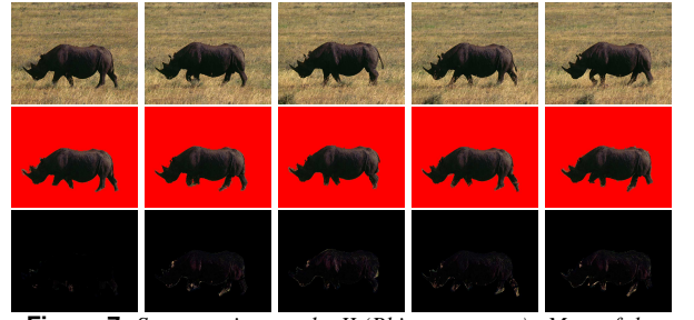
Figure 7. Segmentation results II (Rhino sequence). Most of the errors are due to a part being partially occluded by the background.
