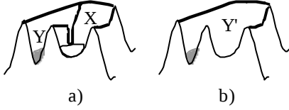
Figure 5: Removal of basin X in Figure 4a by digging. a) generation of a vertical crack in the watershed line from point LO_{XY} to the regional minimum of X; b) watershed transform after digging transformation.
