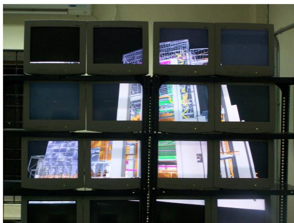
**Fig. 7.** A 4x4 display wall rendering of UNC's Powerplant. The combined resolution is 12 MPixels. Efficient rendering to a display wall requires fast visibility culling of the scene to all the frustums. Adaptive culling by merging of the object and frustum hierarchies makes this possible for even bigger tile configurations.
