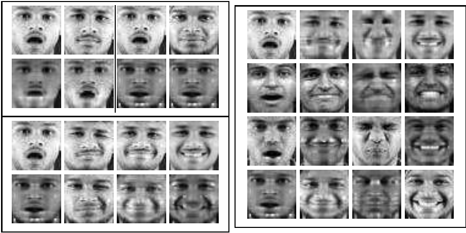
Fig. 7. Results of expression transfer using the algorithm described in section 3. First table : The top row shows frames from the facial expression video and the neutral face video considered for expression transfer (The first neutral face corresponds to the same subject). The second row shows the frames of the synthesized video using the algorithm. The third and fourth rows show four expressions (surprise, wink, smile, giggle ) transferred to the neutral face of another subject. Second table : the expression transfer algorithm on a set of four subjects where the expression in the videos along the diagonal were transferred to other subjects (the columns show the same expression for different subjects and the rows show the same subject in different expressions). Only the diagonal videos were originally available.
