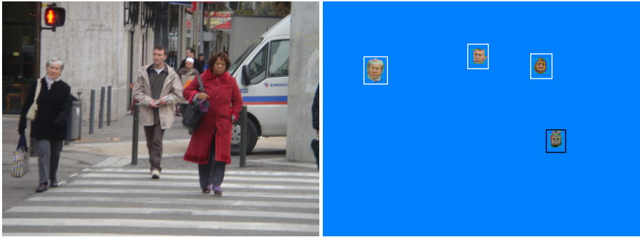
Fig. 4. The figure shows an image from the INRIA pedestrian data set. After running our algorithm, we obtain four face segmentations, one of which (the one bounded by a black square) is a false detection. The energy-per-pixel values obtained for the true detections were 74, 82 and 83 while that for the false detection was 87. As you can see the energy of false detection is significantly higher than that of the true detections, and can be used to detect and remove it.
