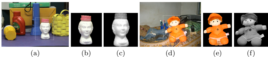
Fig. 11. (a) and (d) Cluttered scenes with user selected ROI. (b) and (e) Extracted object using GrabCut. (c) and (f) Recognized object from IGOIL.
