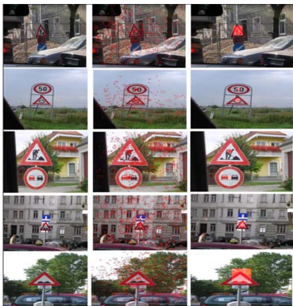
Figure 4: (Left) The test images. (Middle) Clustering of SIFT descriptors at the centre of traffic signs. (Right) Bounding boxes of traffic signs.
