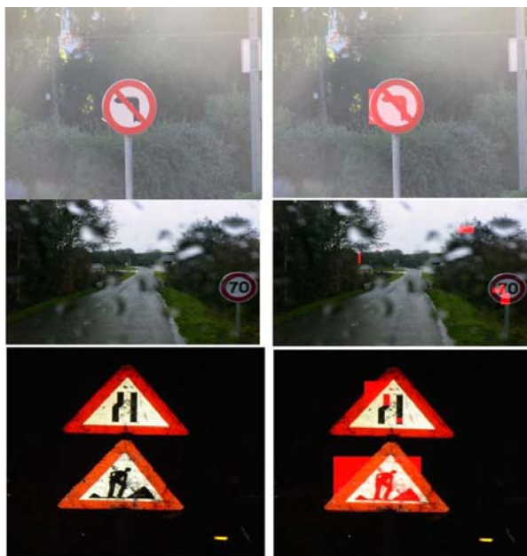
Figure 13: Sample traffic signs and correct detection and classification under different illumination conditions.
