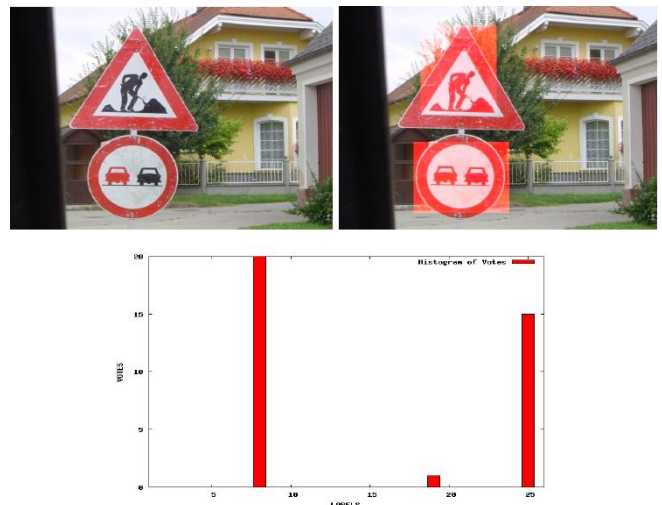
Figure 12: Detection with high threshold ( \tau=5 ).
