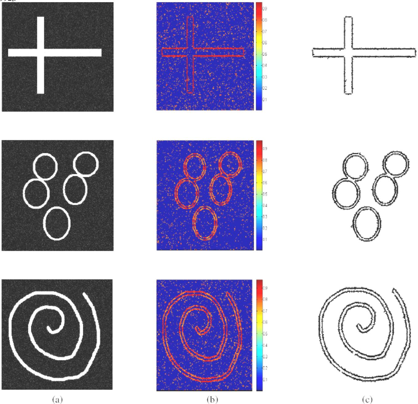
Figure 3. The results of our approach on synthetic image with noise. (a). First column shows the input images with Gaussian noise. (b). Second column shows corresponding DSM. (c). Third column shows the results after post processing.
