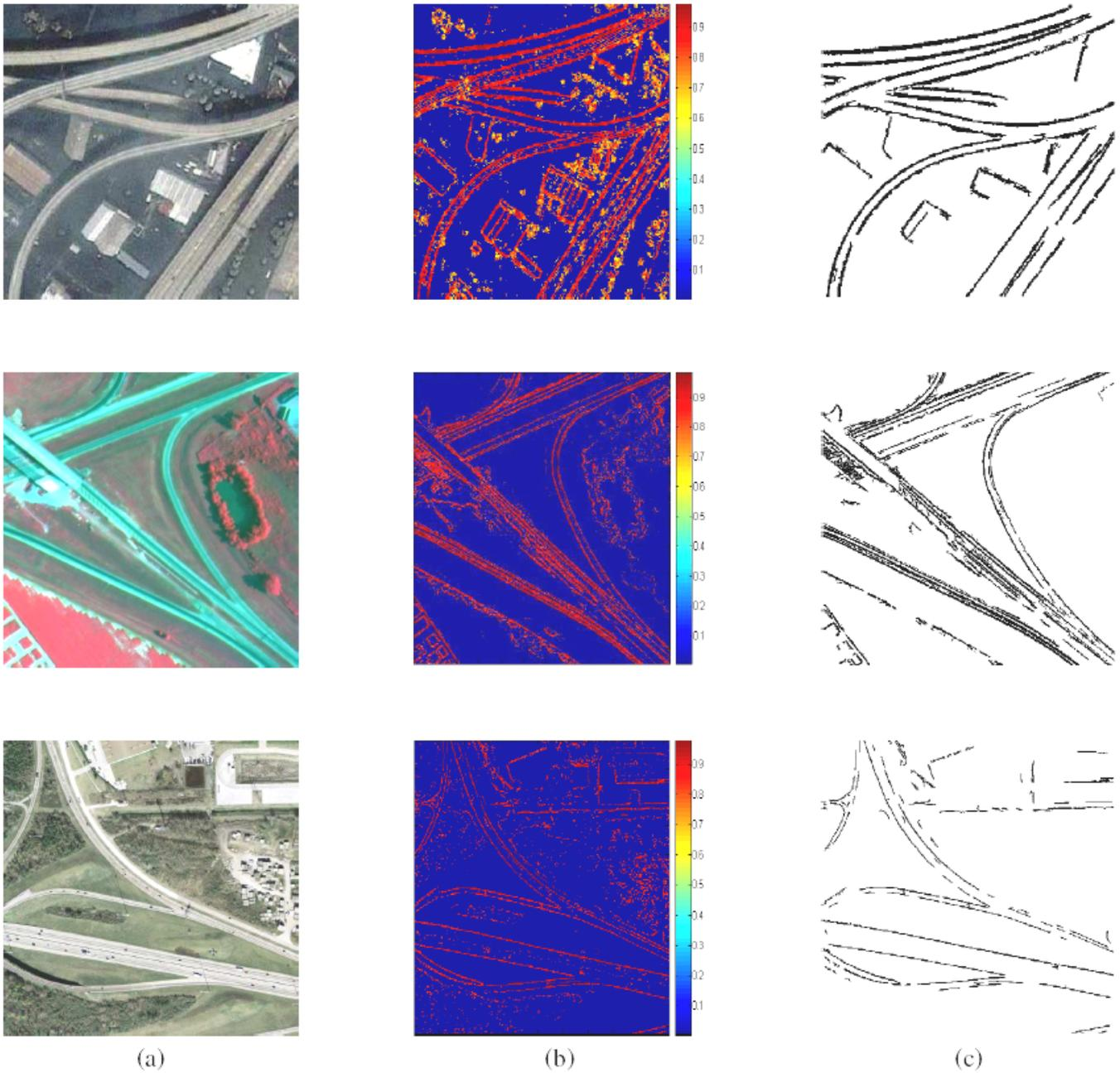
Figure 4. The results of our approach on real-world images. (a). First column shows the input images. (b). Second column shows corresponding DSM. (c). Third column shows the results after post processing.
