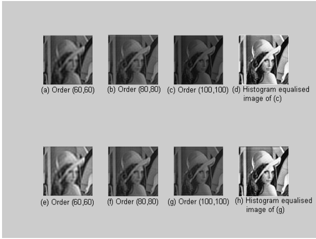
Fig.3. Reconstructed images of Lena with different orders (a)-(d) Legendre moments, (e)-(h) Pollaczek moments.
