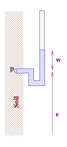
• The total head h(p) is the sum of the hydrological head w(p) and the elevation e(p).
