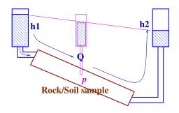
Total head=elevation+hydraulic head h(p) = e(p) + w(p)
